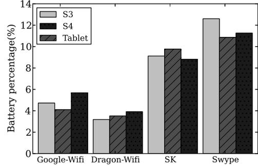
Fig. 6. Battery level consumption for phone and tablet
